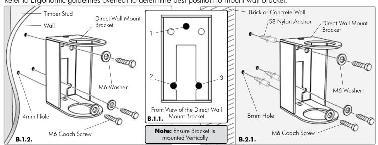
**B.1. For Timber Stud Mounting -** Use the Direct Wall Mount Bracket to mark out the location of the required three holes (see diagram B.1.1.). Drill 3x4mm holes deep enough to receive the M6 Coach Screws, insert the screws and secure the bracket to the wall (see diagram B.1.2.)
